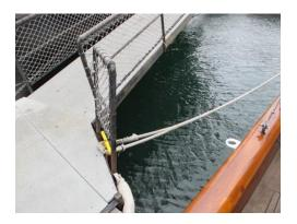
4. Stern Line: Pulled back to dock when we cast off; heaved to boat for docking.
