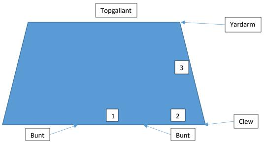
T'gallant: The t'gallant does not have a reef so there are only 3 segments to consider when furling the sail. Segment 1 is addressed like the topsail and is described above. Often the third segment is also addressed at this point by bringing the leech boltrope up to the yard, finding its center and pulling this point inboard as a fold that one traps under the first segment. The innermost gasket on each side is used to secure this part of the sail.
