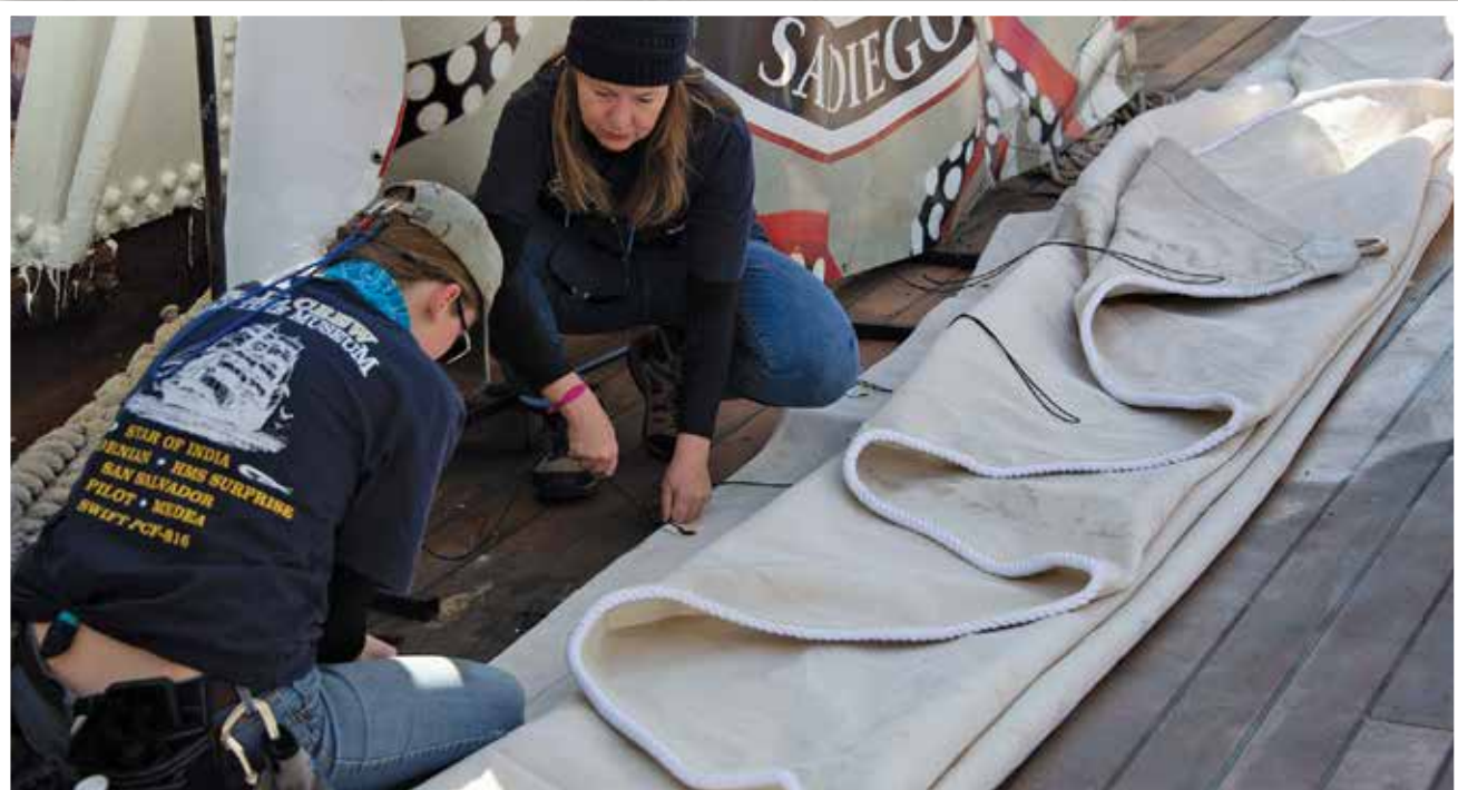
Flaking out the new fore top' mast stay 'sl.
