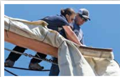
Kaitlyn Porter and John Draper work on an earing lashing.
