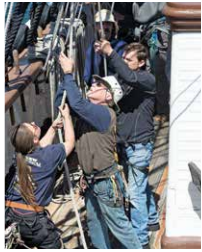
Volunteer crew man the clews bunts and leaches to haul up the newly installed lower top'sl.
